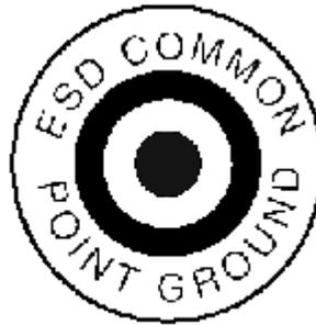
6.2.6.2 Figure 10 shows the universal ESD susceptibility symbol indicating the presence of static sensitive devices, assemblies or systems. This symbol appears on labels and signs to alert personnel of the need for special handling of equipment. Figure 11 shows the universal symbol indicating protection to ESD sensitive devices. This symbol can be used to identify tools, material and equipment that are specifically designed to provide ESD protection.
