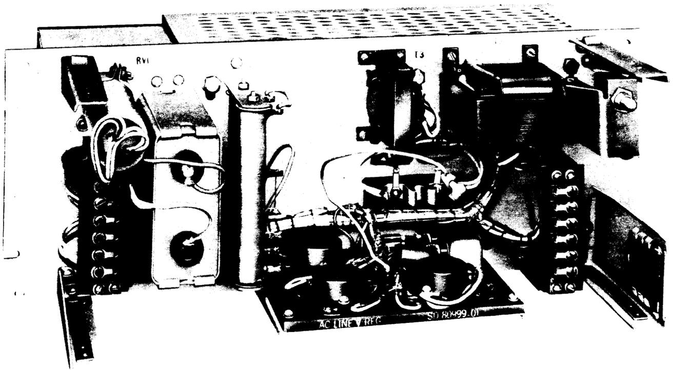
Fig. 3 - Regulator - Rear View
