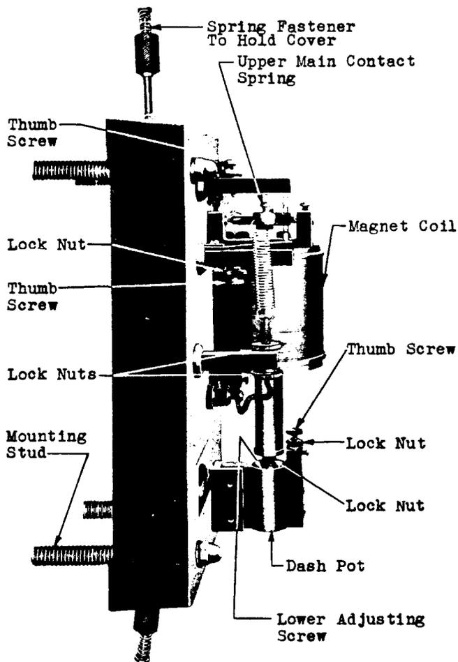
Fig. 2 - Regulator Assembly (Side View)
