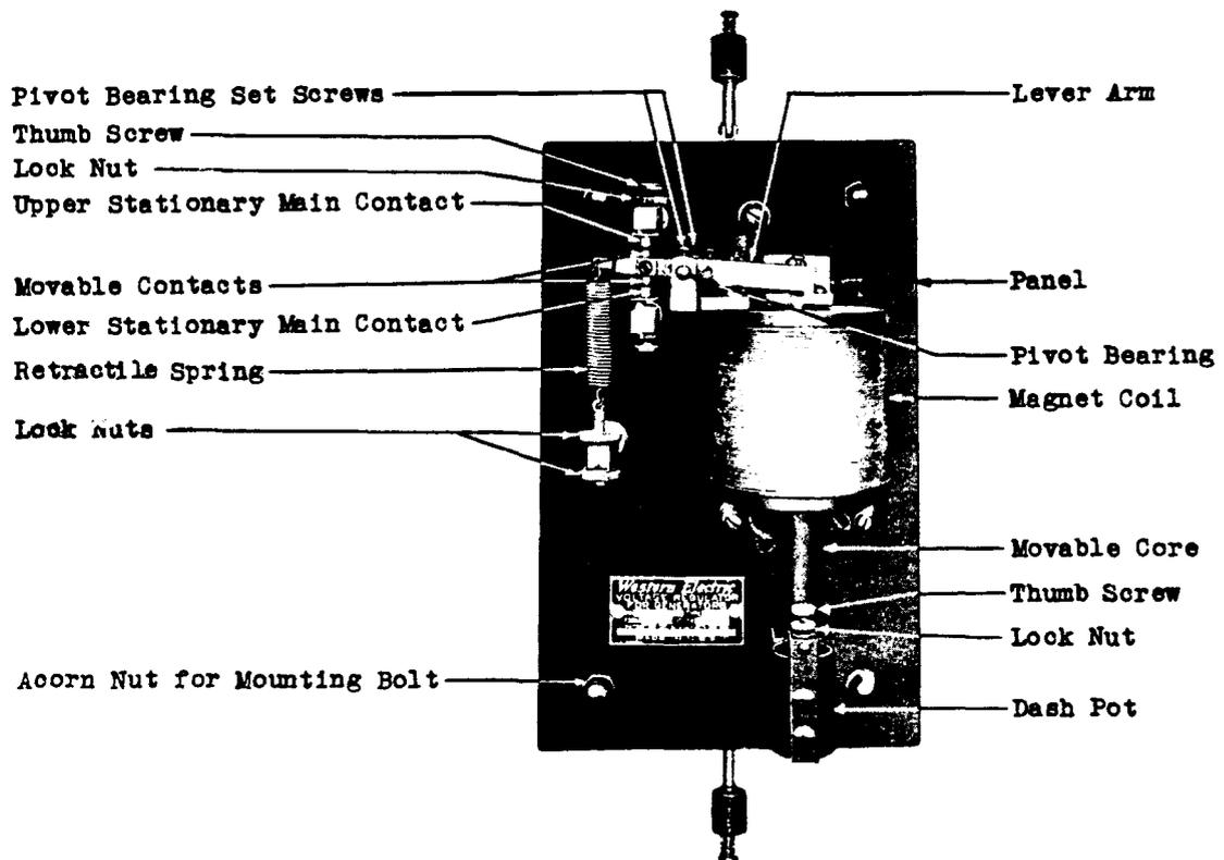
Fig. 1 - Regulator Assembly (Front View Cover Removed)
