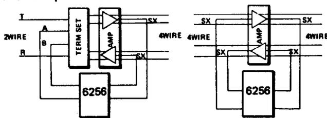
figure 4. 2W/4W and 4W/4W interfaces
