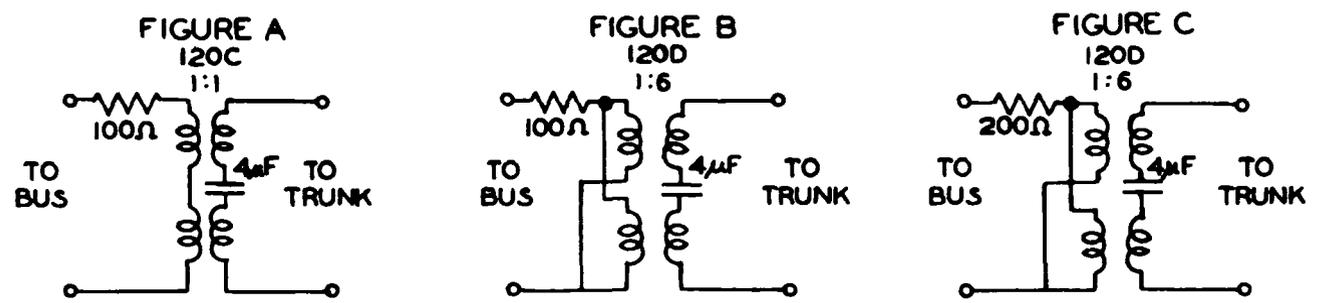
Fig. 4—Equalization of Trunks Between Announcement Bureau and Subcenter
