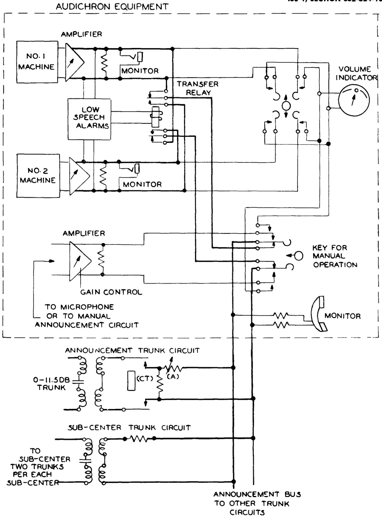
Fig. 1—Time Announcement System 4A — Dual Audichron Machine Transmission Schematic
