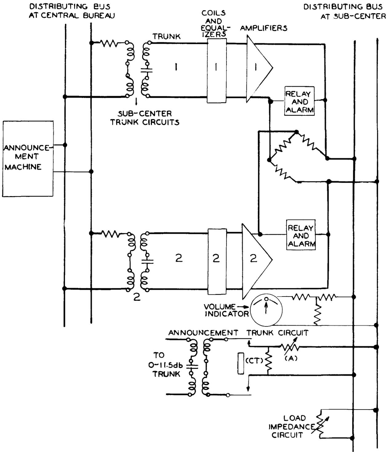
Fig. 3—Time Announcement System 4A — Distribution Through Subcenters
