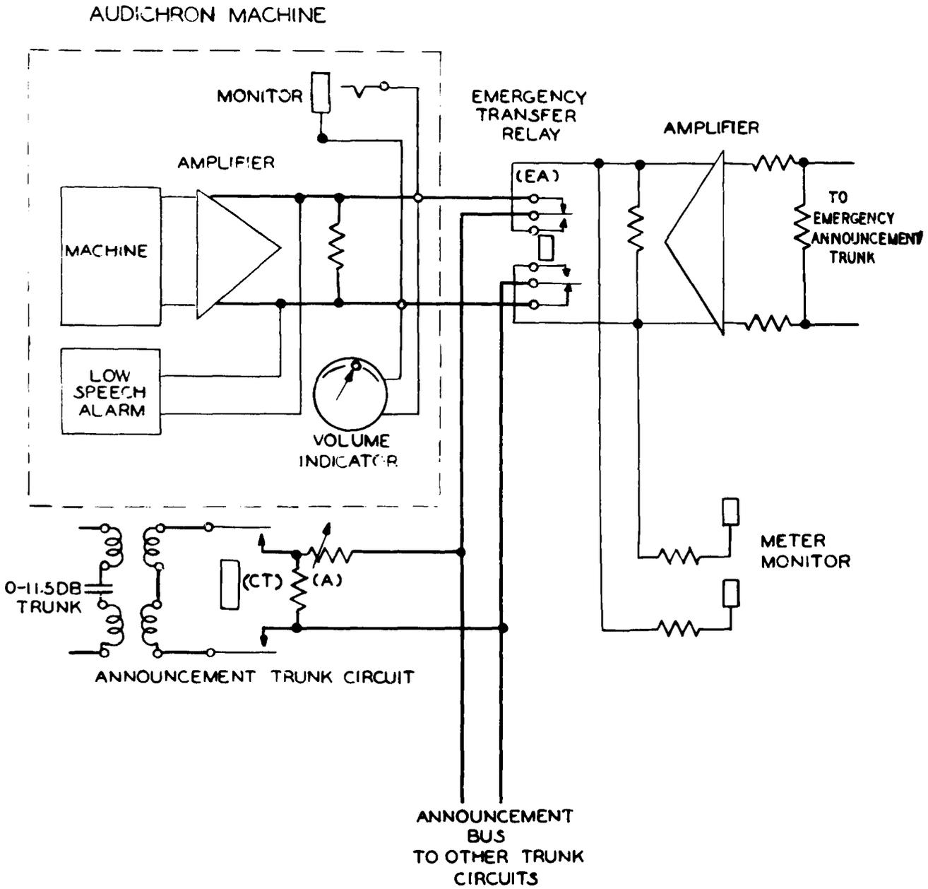
Fig. 2—Time Announcement System 4A — Single Channel Audichron Machine Transmission Schematic
