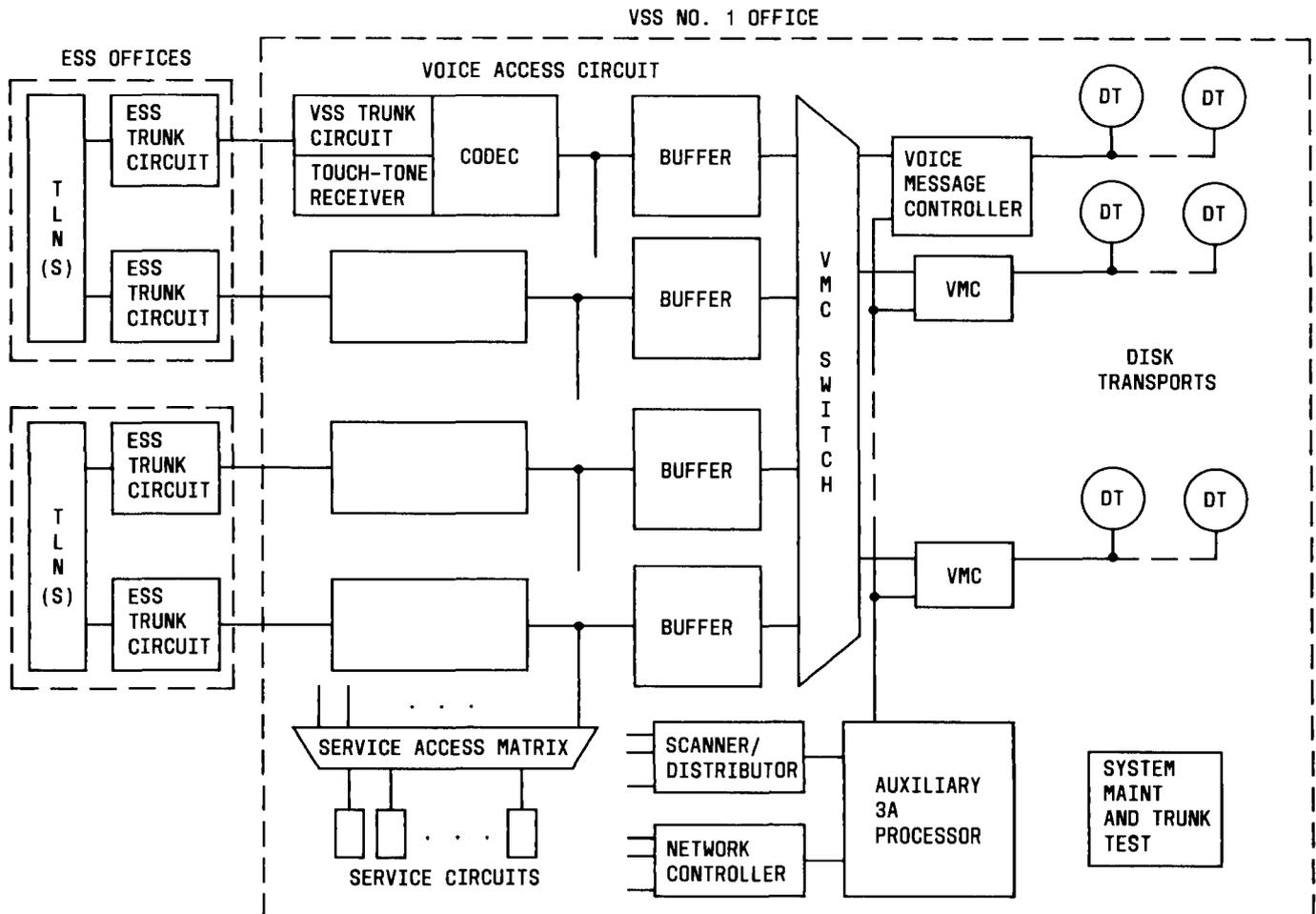
Fig. 1—Block Diagram of Voice Storage System
