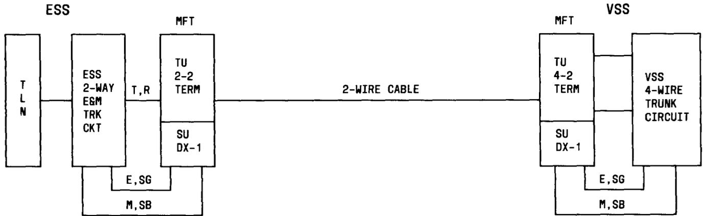
Fig. 7—Typical 2-Wire Metallic Voice Access Trunk
