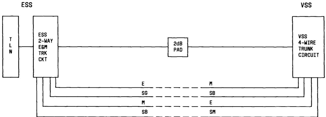
Fig. 8—Typical 2-Wire Intrabuilding Voice Access Trunk
