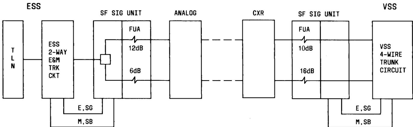
Fig. 10—Typical 4-Wire Analog Carrier Voice Access Trunk With SF Signaling Units
