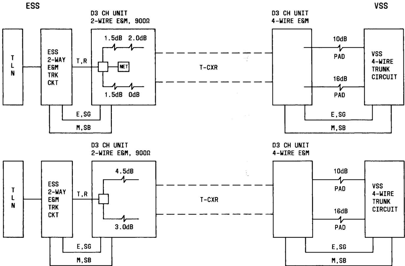
Fig. 9—Typical 4-Wire Digital Carrier Voice Access Trunk With D3 or D4 Channel Banks
