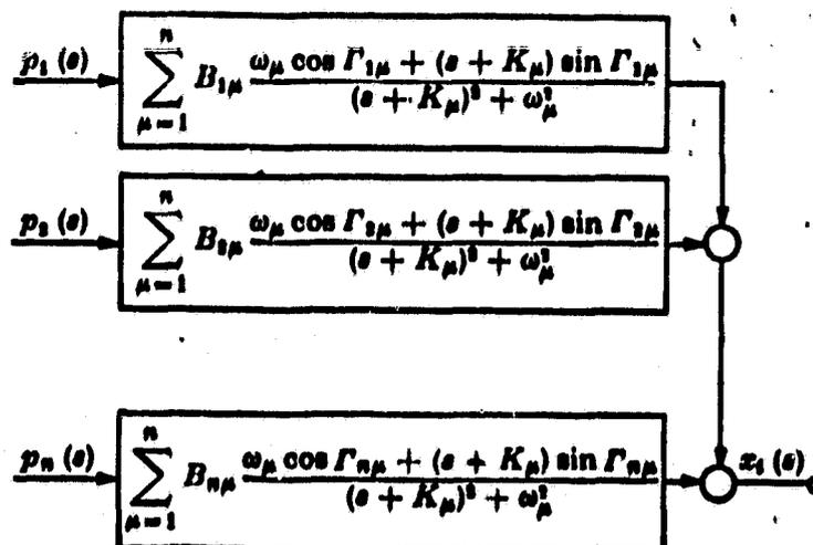
Signal flow chart 3. Transfer function of  $x_1(s)$  according to the Equation (22), for the case when any (arbitrary) excitations affect the structure.
