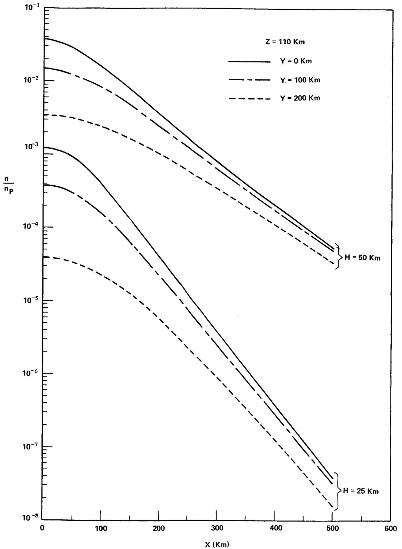
FIGURE 1 - DENSITY VARIATION VS X AT Z = 110 Km IN THE CASE OF A POINT SOURCE
