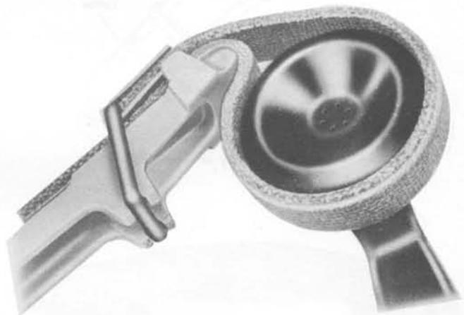
Fig. 2—Correct Positioning of the 514B Tool
