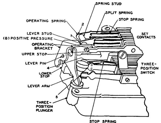
Fig. 3—3-Position Switch (H13 and H14—Type Mountings)
