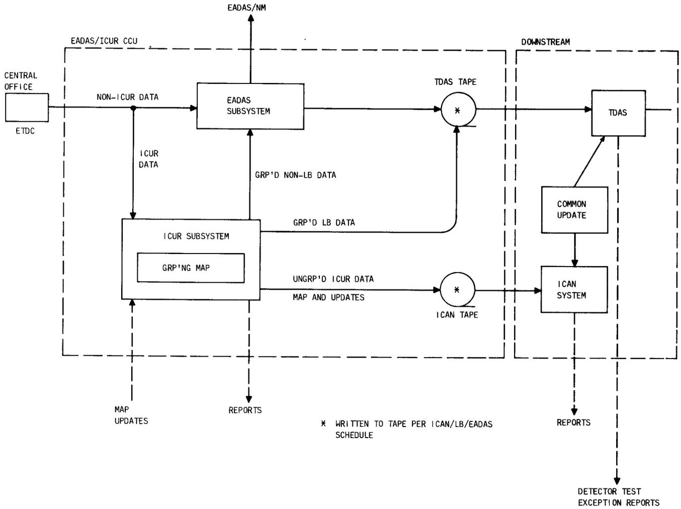
Fig. 1—Simplified Diagram of an EADAS/ICUR System (1.01)
