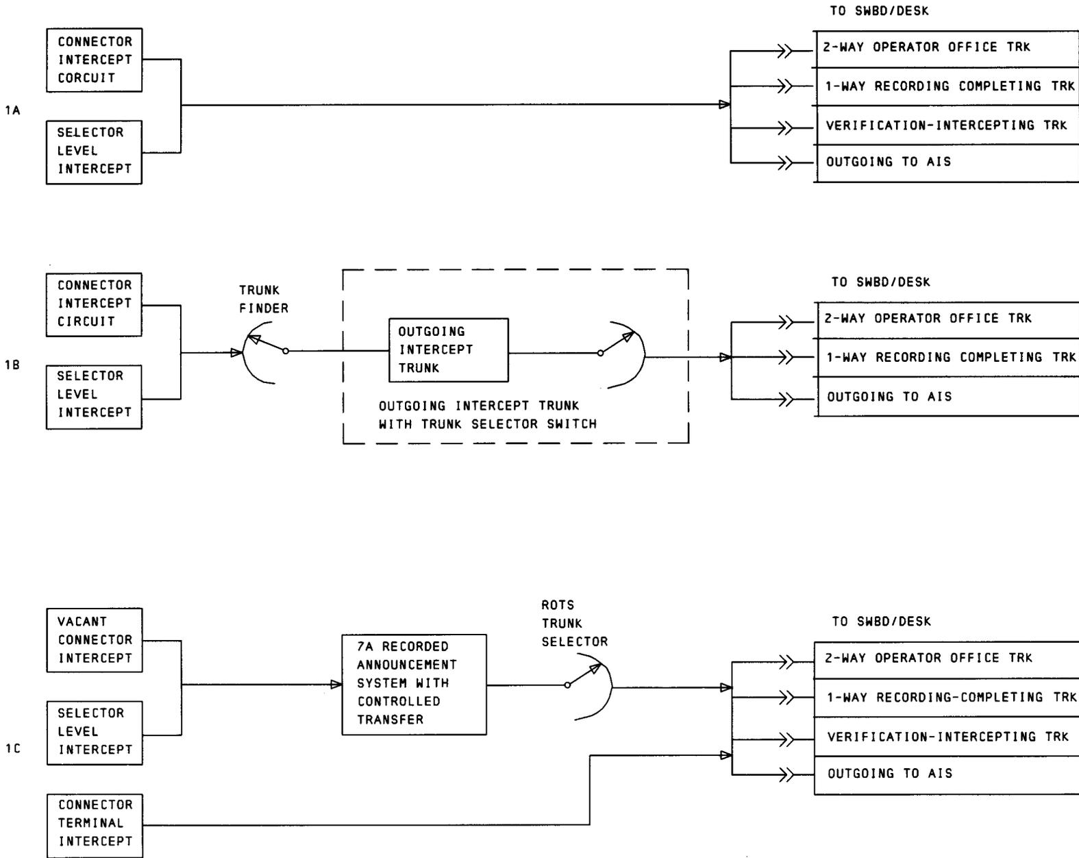
Fig. 3—Intercepting Trunk Arrangements for a Typical 355A CDO (3.08)
