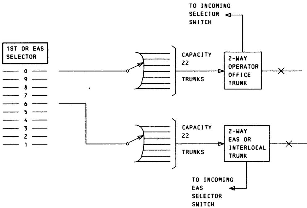
Fig. 4—Typical Out-Trunk Switch Arrangements for Operator Office and EAS Trunk Groups (4.11)
