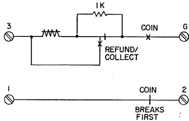
Figure 4. Coin Relay Contact Spring Assembly and Schematic.
