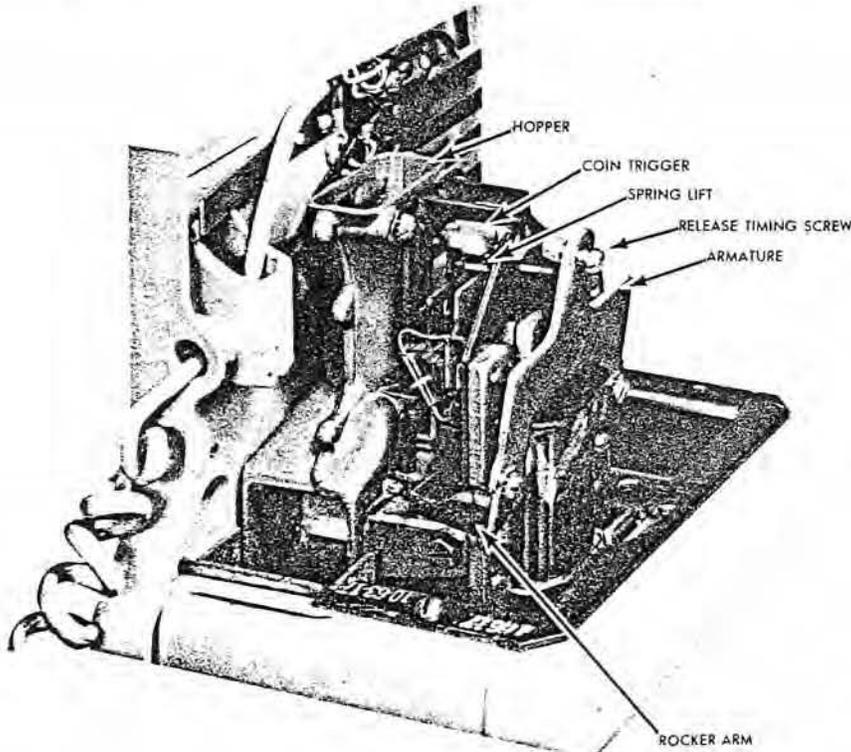
Figure 1. Single-Coil Coin Relay, Shown Installed,
