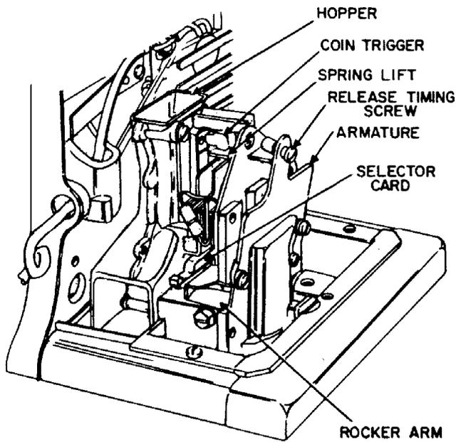
Figure 2. Single Coil Coin Relay, Installed, Cover Removed.
