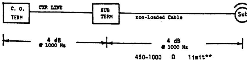
\* IF LESS THAN 0.4 LOAD SECTION, BUILD OUT TO ½ LOAD SECTION.
