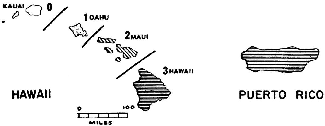
Fig. 3 - Map for Seismic Zones-Hawaii, Alaska, and Puerto Rico
