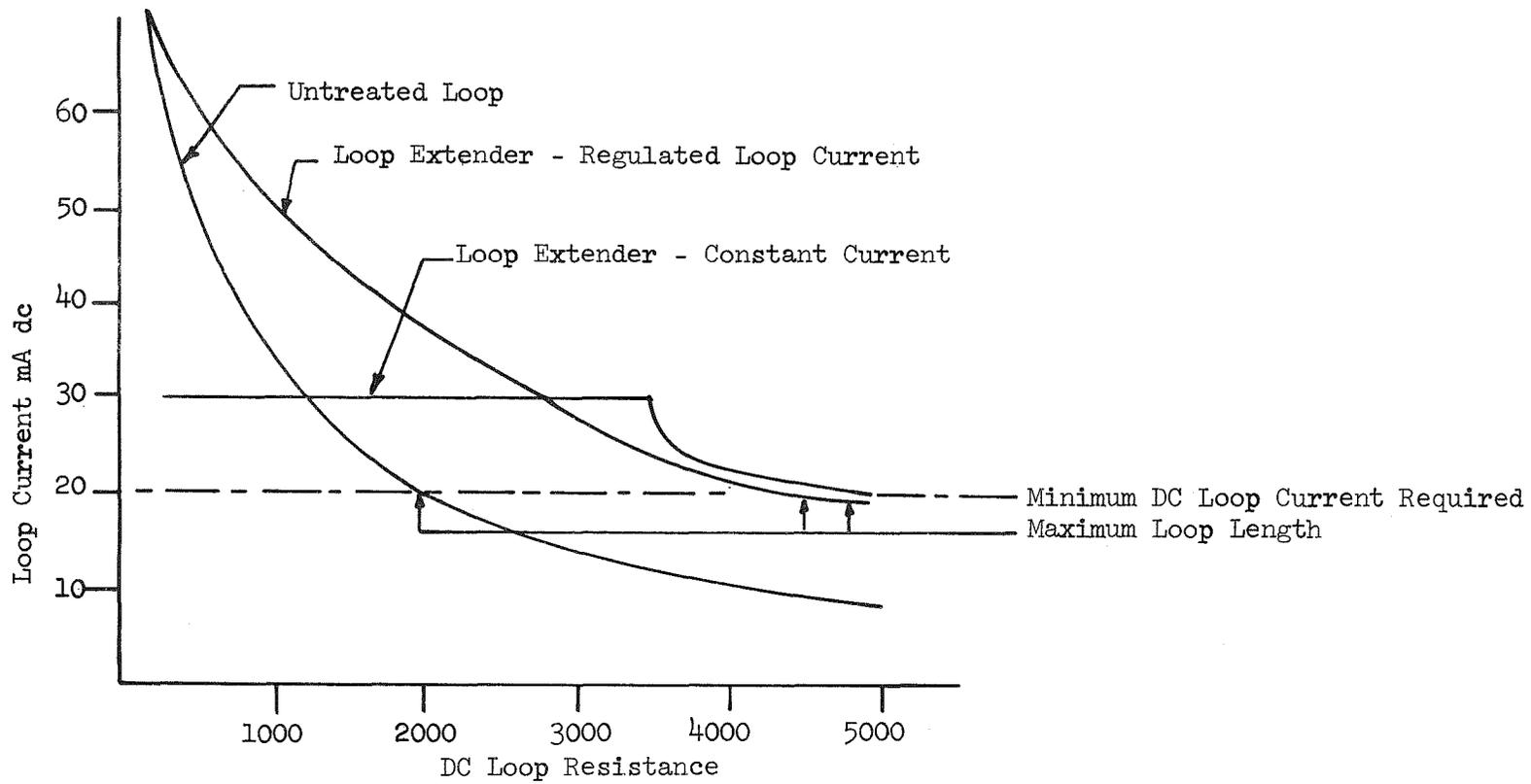
FIGURE 2 Loop Current vs Loop Resistance for Loop Extender Equipment
