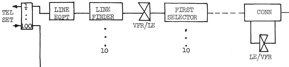
FIGURE 3 Typical S x S Switch Path With CMO
