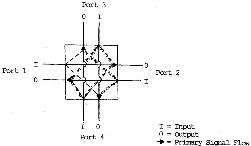
Figure 6 Four-Way, 4-Wire Bridge
