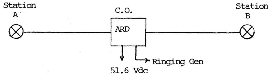
Figure 10 Typical Ringdown Circuit
