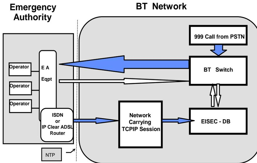
Figure 1 Service Schematic
