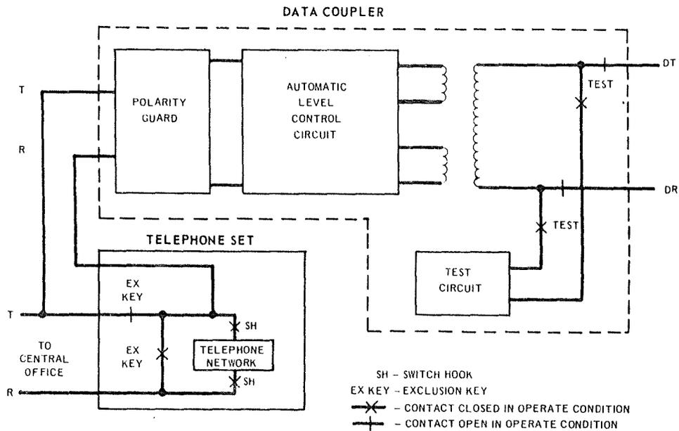
FIG. 4 - DATA ACCESS ARRANGEMENT CDT
