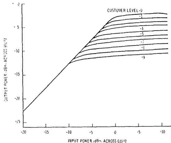
Fig. 5 - Limiting Characteristics of the 1000A Data Coupler
